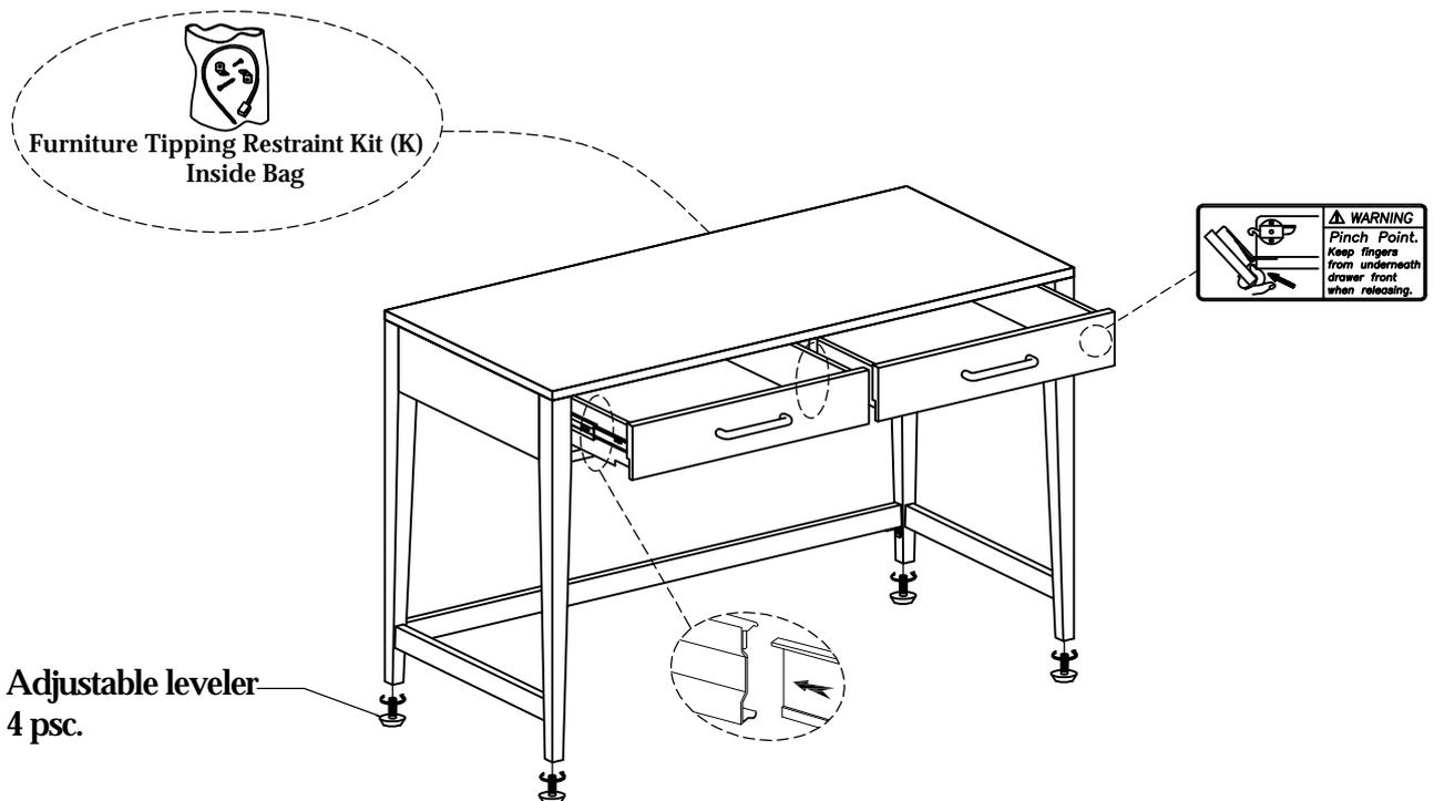
For product and personal safety, a Furniture Tipping Restraint kit has been included with this unit which can help to minimize the risk of the unit accidentally tipping forward, if used and properly installed per the kit manufacturer's instructions.
